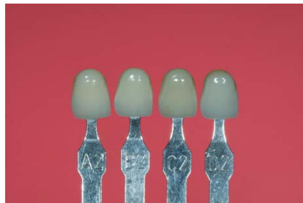
Figure 11: Dental shade tabs in front of an illuminated pink background (simulating gingiva) were captured by a camera with white balance set to “Auto.” The camera sensed the high proportion of reddish color in the scene and added cyan to neutralize the image. The color of the shade tabs was simultaneously modified and inaccurate.
