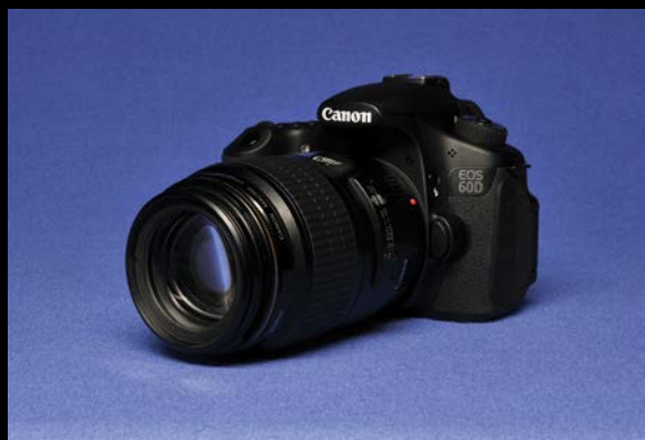
Figure 2: Moderately priced Canon camera model with corresponding Canon 100mm macro-style lens mounted in place. Although designed in different positions than competing Nikon cameras, this model also comes with separate shutter speed and aperture control wheels to easily dial in the desired manual exposure setting.
