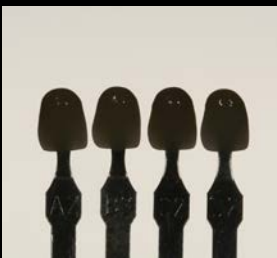
Figure 8: Dental shade tabs in front of an illuminated white background were captured by a camera in aperture priority (automated TTL) exposure mode. The camera sensed the high proportion of light tones in the scene and underexposed the strobe lighting of the subject.
