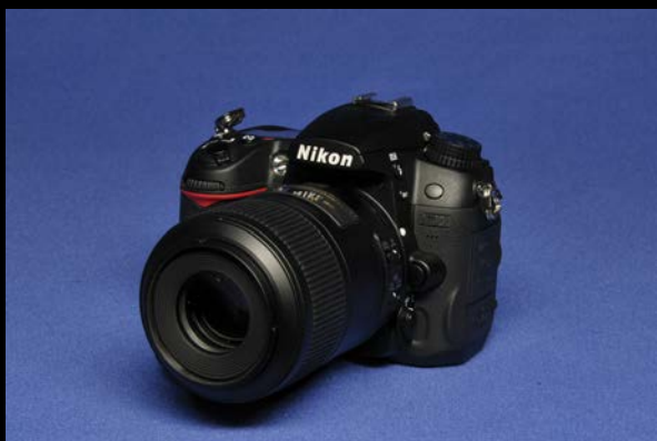
Figure 1: Moderately priced Nikon camera model with corresponding Nikkor 105mm macro-style lens mounted in place. This example has separate shutter speed and aperture control wheels to easily dial in the desired manual exposure setting.
