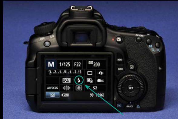
Figure 14: Most contemporary DSLR camera bodies display confirmation of the current white balance setting in a window on top of the camera or in an information display on the back. (See the lightning bolt icon representing the “flash” setting in the center of this image.)
