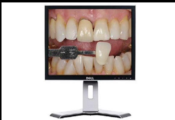
Figure 4: This example of a high-end 4:3 aspect ratio computer display has 1600 x 1200 pixels (totaling only 1.92 megapixels). High-definition displays have 1920 x 1080 pixels (totaling only 2.07 megapixels). Additional pixels exceeding these totals would not be displayed.
