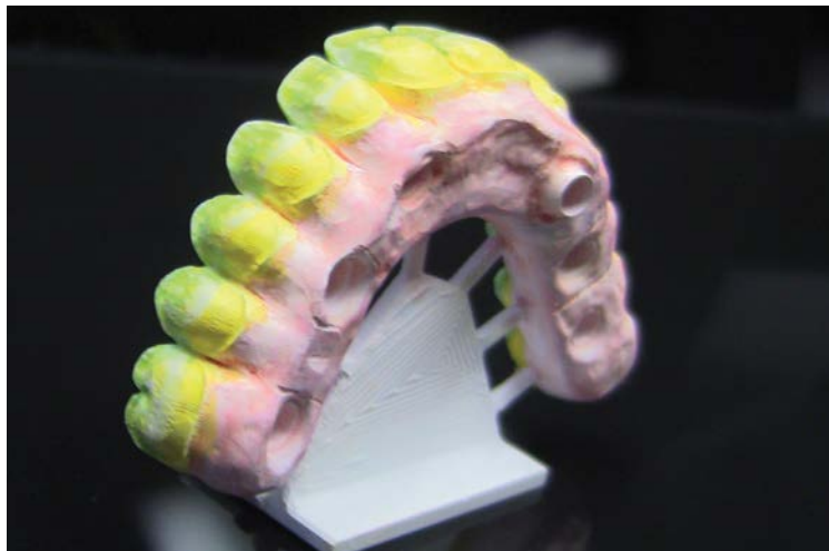
Figure 19: Zirconia was stained in the green stage with an acid-free water based color liquid.
