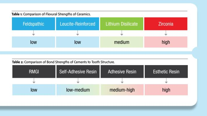
When using a high-strength ceramic, such as zirconia, with a retentive preparation, low-strength cement such as a self-adhesive resin cement or RMGI can be used because it is not necessary to rely on the cement for additional strength.<sup>6</sup> **Table 1** compares the strength of all-ceramic restorations and **Table 2** compares the bond strengths of different classes of cements.
