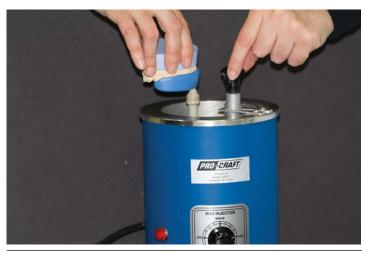
Figure 9: Wax injector.
