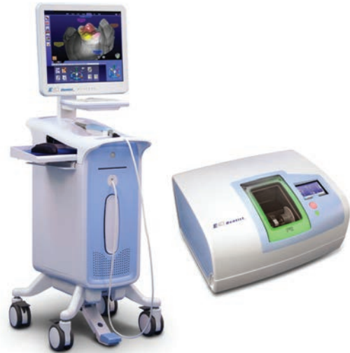
Figure 2: E4D Design Center and milling unit.
