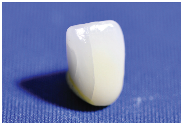
Figure 2: This veneer was intentionally cooled too quickly to dramatically show this problematic characteristic of porcelain.
