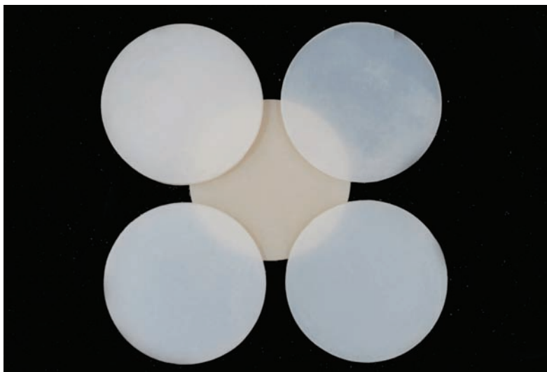
Figure 7: ENA HRi UE2 enamel samples with increasing thickness over a sample of UD 3 dentin. The ENA HRi enamel, with a refractive index of 1.62, demonstrates optical behavior similar to natural enamel. Increasing the thickness also increases the value.
