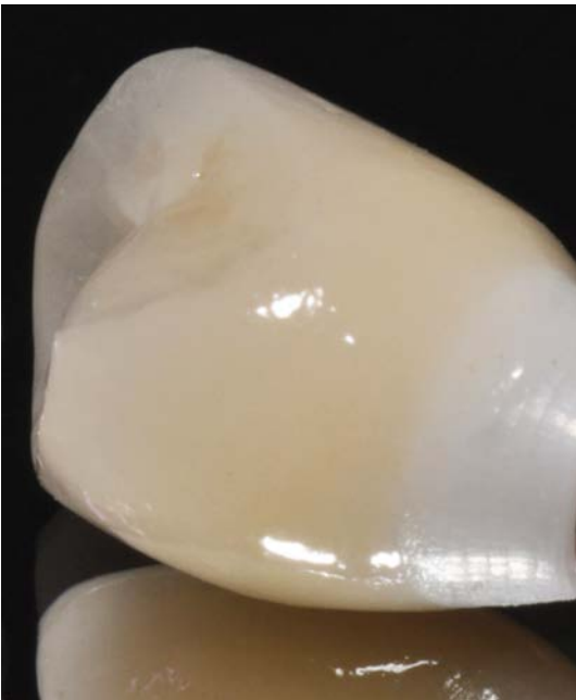
Figure 12d: Chipping fracture: cohesive failure of veneering porcelain.
