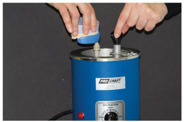
Figure 9: Wax injector.
