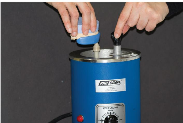
Figure 9: Wax injector.
