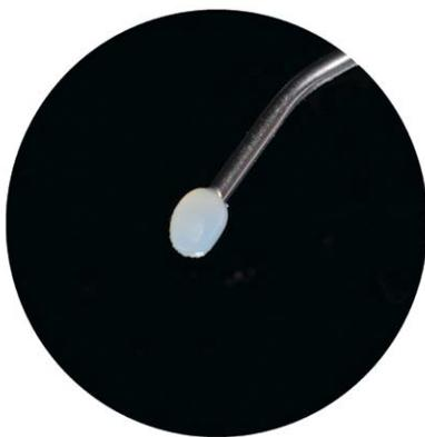
**Figure 3:** Opal effect material exhibiting bluish appearance under reflected light.
